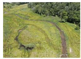
After construction high velocities were reduced as a result of reestablishing floodplain connection, the creation of oxbow wetlands, and microtopography grading with the floodplain.
