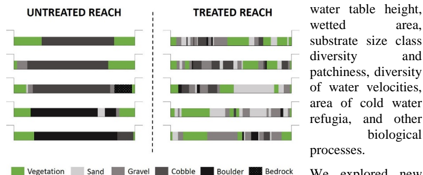
Figure 6: Sediment size class breaks across valley-wide transects - 5 transects in the untreated reach and a sample of 5 from the treated reach. This depicts visually the difference not only in substrate size, which is much finer in the treated reach, but in substrate diversity and patchiness, which has important ecological implications.
