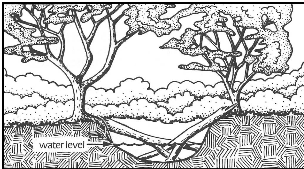
Figure 7. Condition 2 large woody debris structure (AFS, 1983).
