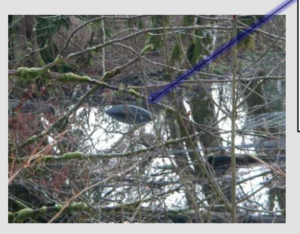
Note elevated pipe. This installation was a failure because the pipe was not anchored down securely in the section passing through the dam. Beaver, in their predicted repair of the dam breach, inadvertently lifted the pipe, thus defeating the effectiveness of the bypass installation.
