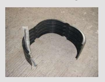
It is sometimes necessary to cut the 20' lengths into 10' length for ease of transport. Pipe sections are easy to join/rejoin with couplers.
