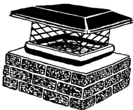
Fig. 6. A cap or exclusion device will keep raccoons and other animals out of chimneys. These are available commercially and should be made of heavy material. Tightly clamp or fasten them to chimneys to prevent raccoons from pulling or tearing them off.
