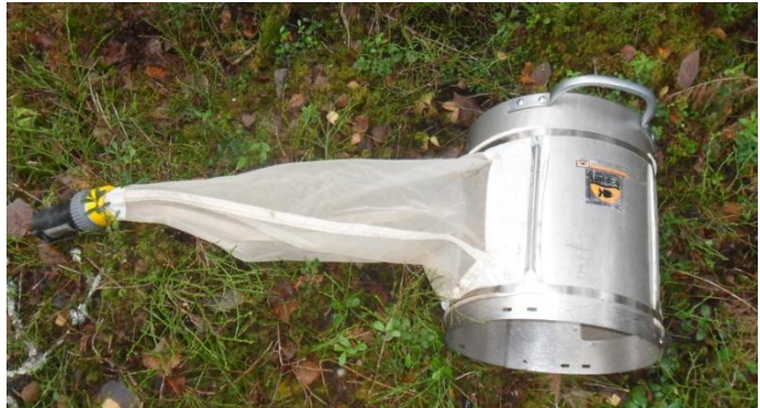
Fig. 3. Hess sampler used for sampling of macroinvertebrates in streams with a sandy/rocky substrate.
