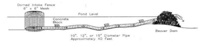
In order for these pipe systems to be effective, they must be designed so that beavers cannot detect the flow of water into the pipe. The Flexible Pond Leveler™ does this by surrounding the submerged intake of the pipe with a large cylinder of fencing which is placed in as deep water as possible. This prevents the beavers from detecting the flow of water into the pipe. As a result, the beavers do not try to clog the pipe, and a safe water level can be maintained.
