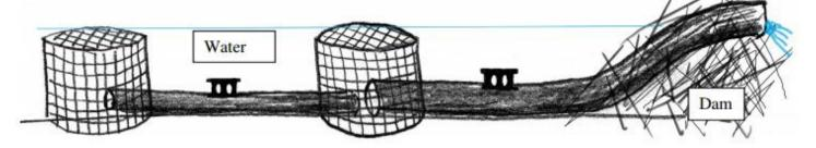
The "Ditch Leveler"™ design is based on the highly successful Flexible Pond Leveler™ which has been successful in thousands of locations. The Ditch Leveler™ is intended specifically for use in deep, <a href="mailto:narrow">narrow</a> channels where there is not room for a large exclusion cage. It spreads the flow into the pipe over multiple areas so smaller exclusion fences can be installed in the narrow channel. See diagram.
